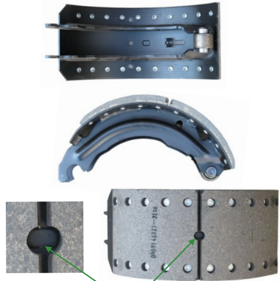
Brake shoe with cut out in the lining and a small locating key on the brake shoe
