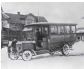
The so-called "Nordmark" bus was the first entirely Swedish-built omnibus. Built by Scania in Malmö in 1911 on a truck chassis, it was fitted with an engine and body at Vabis in Södertälje, Sweden.
