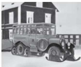
Motor vehicles found it difficult to cope with wintry road conditions. Scania-Vabis constructed fifteen motorised mail buses in collaboration with the Swedish Post Office (1922-23). The first models were fitted with track drives and forward-mounted snow runners, enabling them to be used when the road was completely snow-covered.
