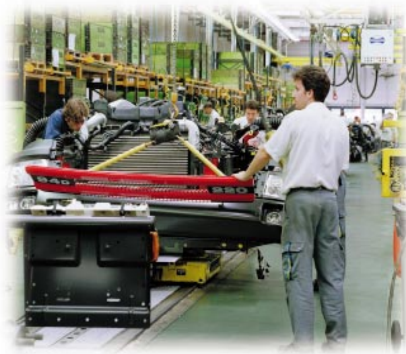
Chassis assembly at Scania's production unit in Angers, France.
