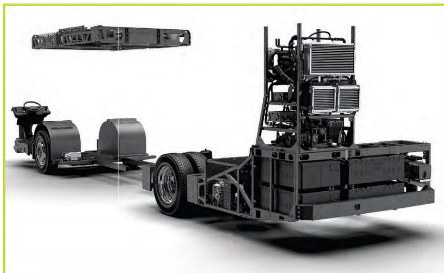
**S**cania has imported its first consignment of Battery Electric Vehicle bus chassis which are currently being built-up by local bodybuilders.
